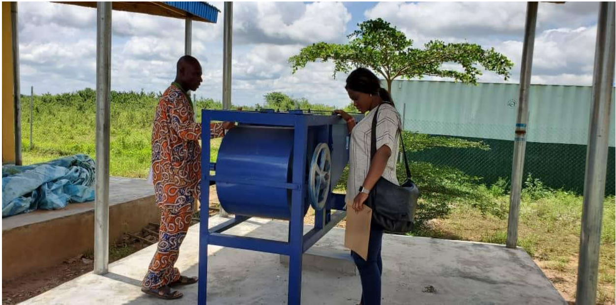
Plates 2: De-Stoning Machine used to remove stones from the rice at by IFAD-VCDP Rice Processing center in Yewa North, Ogun state
