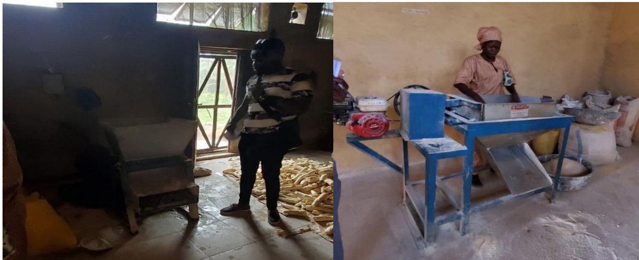
Plates 3: Mechanical Grater and Sieving machine constructed by IFAD-VCDP at Agbelere Baara Cassava Processing center in Obafemi Owode, Ogun state
