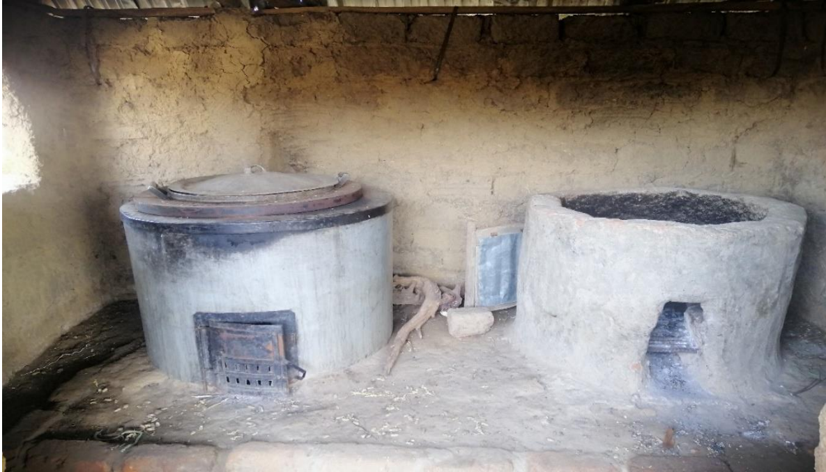
Fig 1.3: False Bottom Parboiling technology built by IFAD-VCDP used for Rice Processing in Kuta, Shiroro LGA, Niger State.
