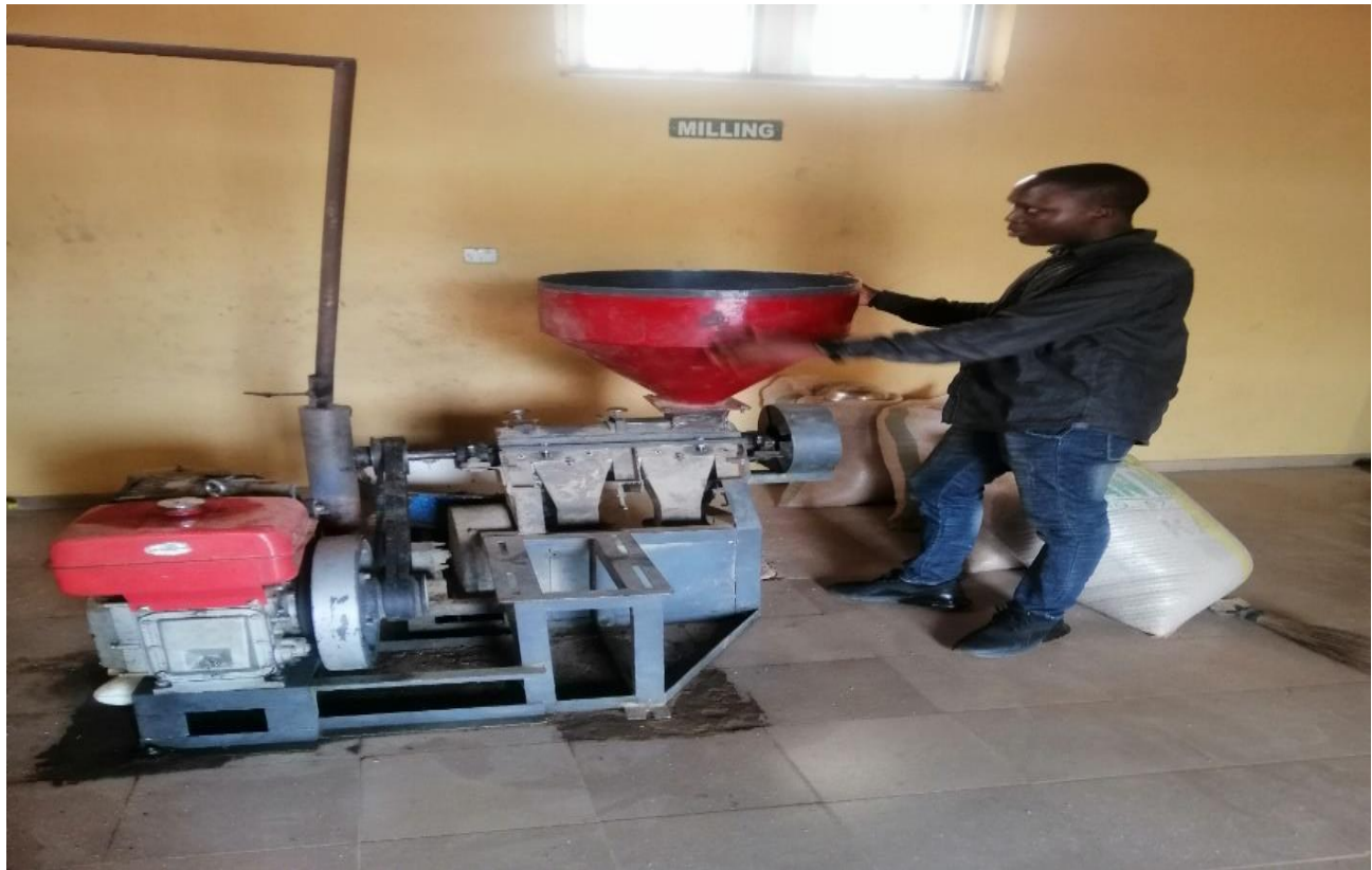
Fig 1.1: Researcher checking the Rice Milling Machine at IFAD-VCDP Rice Processing Plant in Kuta, Shiroro LGA, Niger State.
