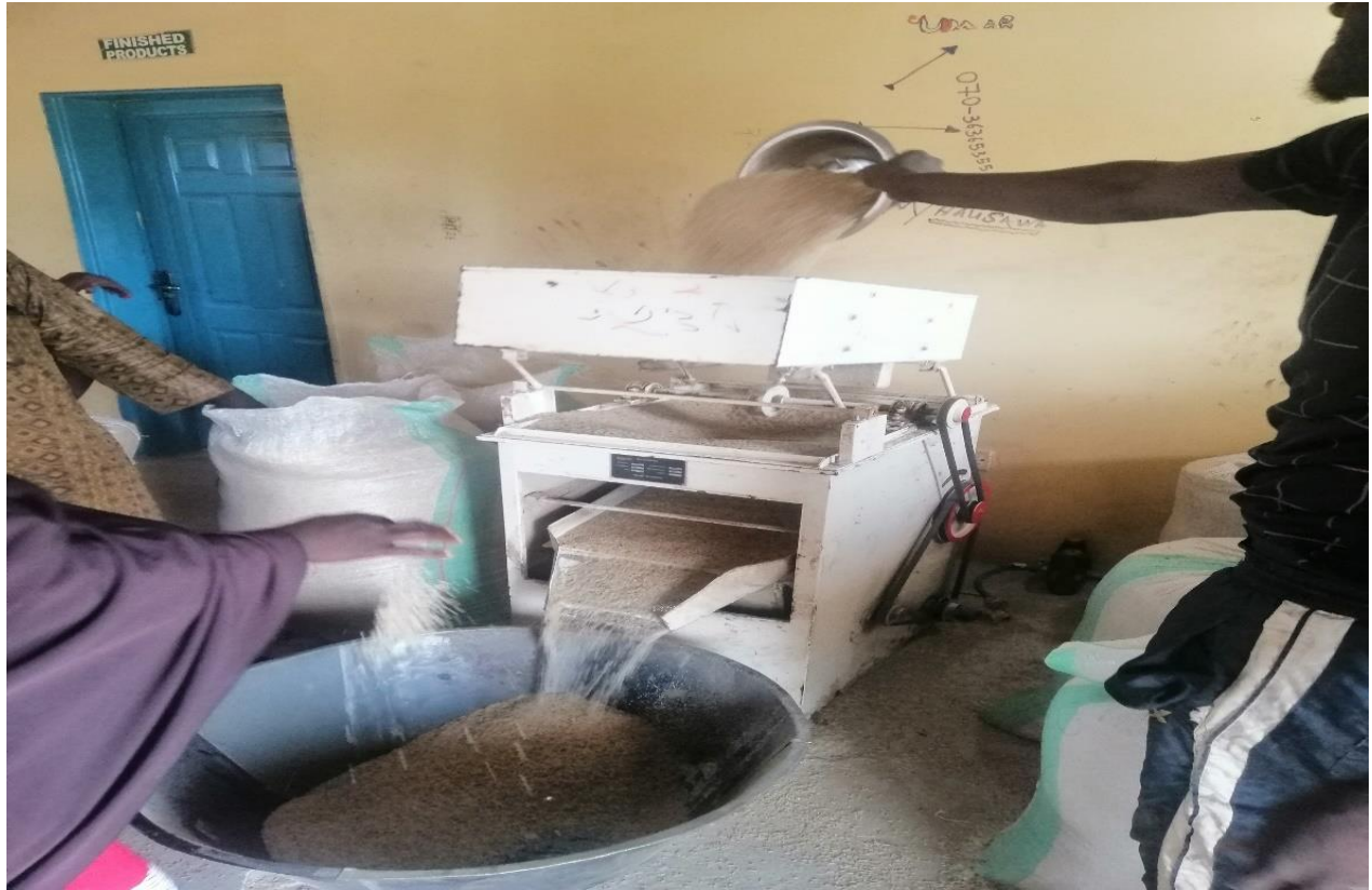
Fig 2.5: Destoner machine used to remove stones from rice inside the IFAD-VCDP Rice Processing Plant in Argungu, Kotangora LGA, Niger State.
