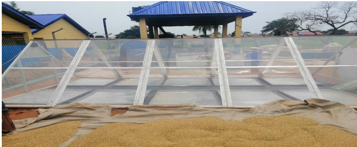
Fig 1.4: Solar Sun dryer machine in the IFAD-VCDP Rice Processing Plant in Argungu, Kotangora LGA, Niger State.
