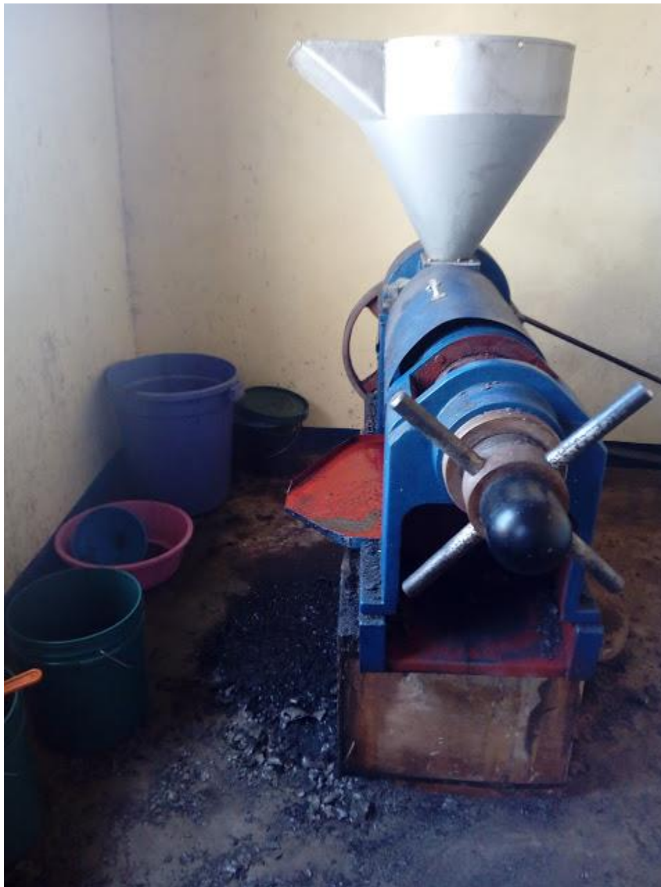
(C) An oil extracting machine used in the Msange Village. (photo by author)
